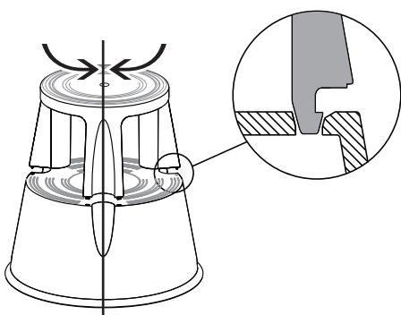
Align the upper part over the lower part, so that the hooks of the legs of the upper part reach into the holes in the lower part.
