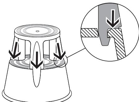
Press the upper part onto the lower part until the hooks of all three legs click into place. Make sure no gap is left between the legs and the lower part.
