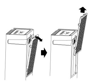
The air filter is removable for easy cleaning. A clean filter helps remove dust, lint, and other particles from the air and is important for best operating efficiency. Check the filter every two weeks to see whether it needs cleaning.
