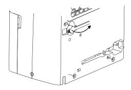
3. Attach a garden hose to the drain hose connector behind the dehumidifier. Securely attach the hose to the root of the drain hose connector, be sure there is no water leak.
