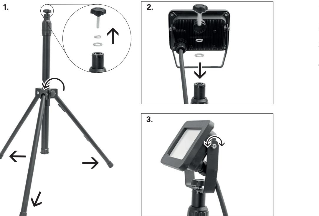
1. Spread the base **8** open and fix it in the desired height with the fixing screw **3**. Remove the fastening screw **1** and its washers from the tripod **10**.
