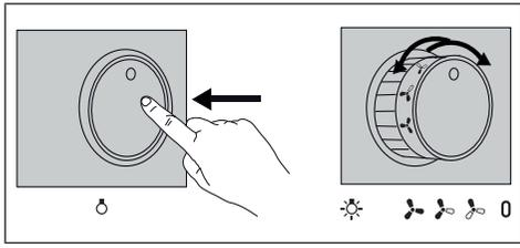
**Lights** - To turn the lights on, press the dial and release it so that it pops out of its housing. To turn the lights off, push the dial back inwards, returning it to the off position.
